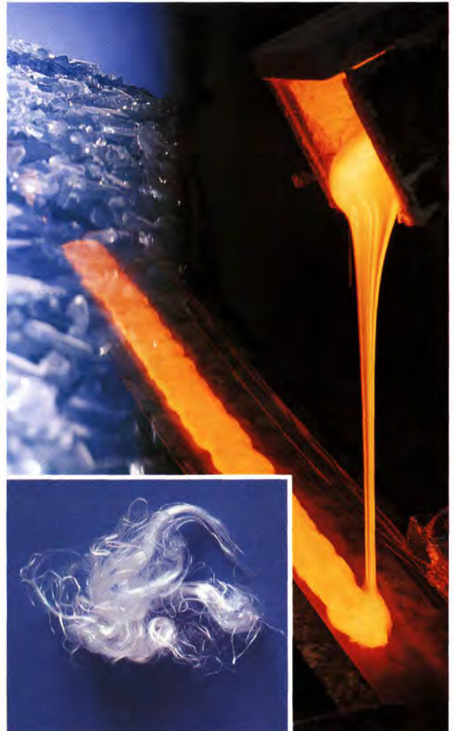
Silica fibers with high thermal resistance (up to 1,100°C) developed by Enka offer interesting prospects.
