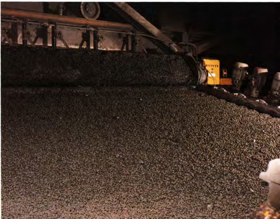
The use of Peridur®, an organic binder for making fine iron ore into smooth pellets, brings energy savings in blast furnaces. The photo shows an ore pelletizing plant in Minnesota (United States).
