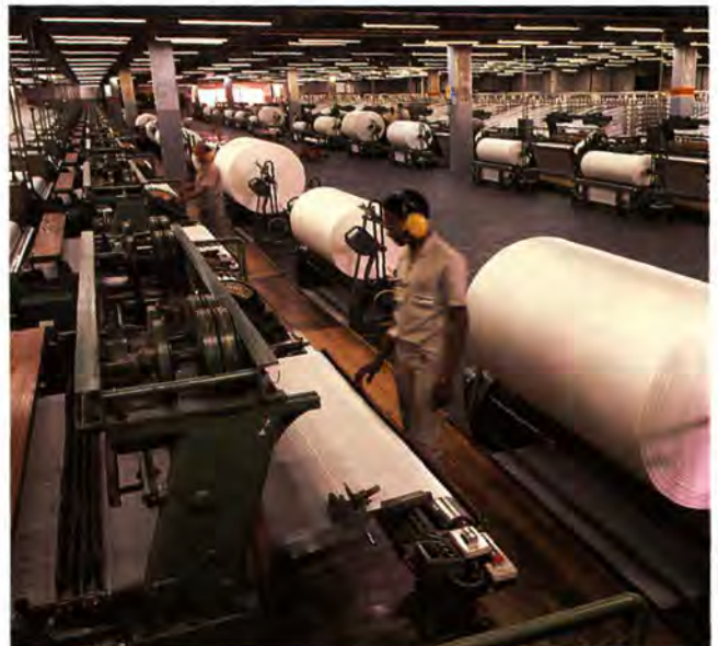
Production of polyamide tire fabric at COBAFI in Camaçari (Brazil). This company has also commenced production of polyester yarns and fabrics.
