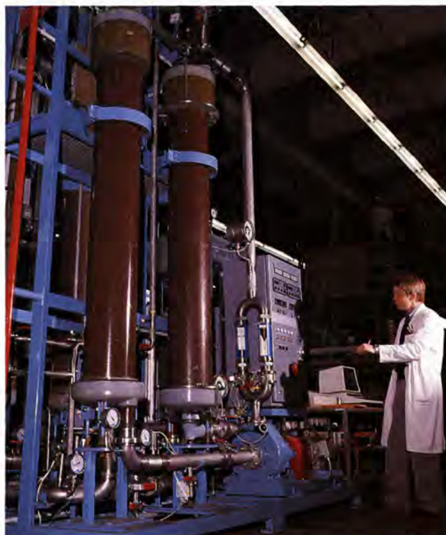
Enka's Trans Membrane Distillation process is used to concentrate aqueous solutions by means of Accurel ® membranes that are permeable to water vapor. The process is based on temperature differences.
